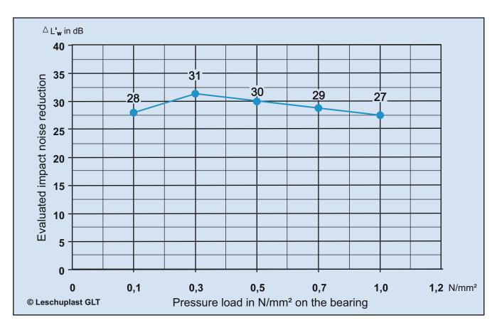
The Leschuplast GLT SD-ribbed bearing can be used in a wide pressure load range from 0.1 N/mm<sup>2</sup> to 1.0 N/mm<sup>2</sup> due to excellent sound absorption properties. In this case, evaluated impact noise reduction of **at least 27 dB** is achieved. An evaluated impact noise reduction of 31 dB is attained with an optimum design at a pressure load of 0.3 N/mm<sup>2</sup>.
